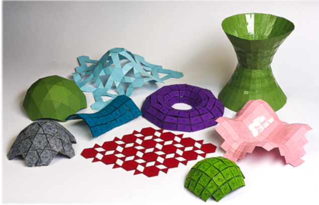
Fig. 18. Photo of all fabricated results deployed from flat, hole-free tilings, constructed from paper or felt and secured with tape.
